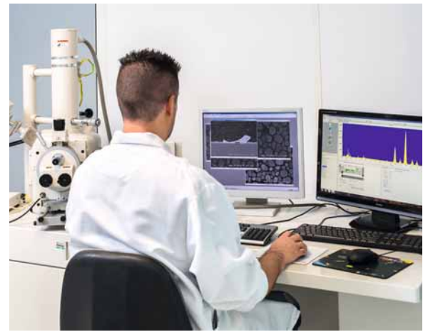
Material analysis of components using an electron microscope and X-ray technology.
