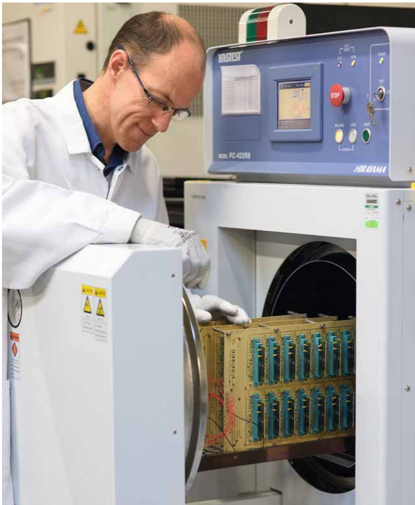
Plastic components are exposed to heat and humidity in the HAST test.
