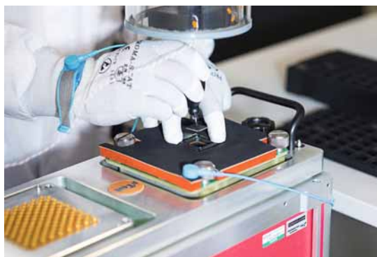
Electronic memory components have to withstand temperatures ranging from -55^{\circ} to +125^{\circ} C.
